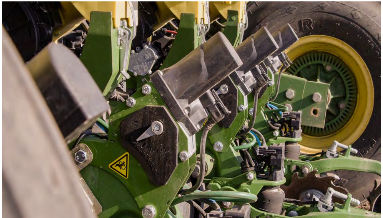
Figure 4. SmartDepth® Control System
