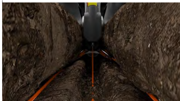
Figure 2: FurrowJet® Dual-Band Wings Fracturing Side-Walls
