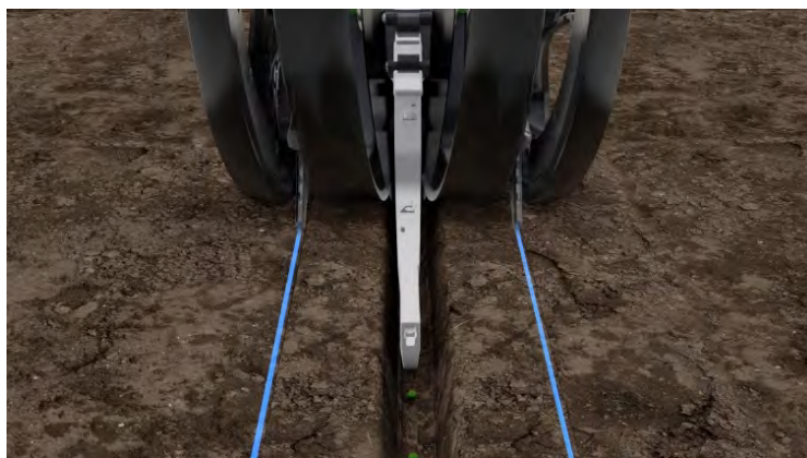
Figure 3. Conceal Dual Placement 3" from Seed
